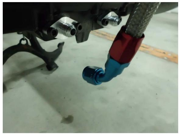
26) A/N fittings are designed to seal via the taper seat in each fitting and <u>NO</u> Teflon tape or pipe dope should be used on the threads. <u>The use of Teflon tape or will promote over-torque of the fitting resulting in damage.</u>
