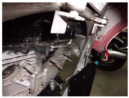
12) Mount the cooler to the frame via the lower mounting bracket using the 10mm hex bolt removed from this location earlier.
