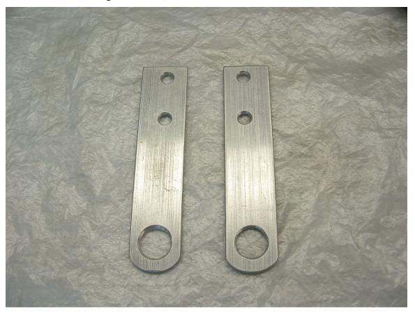
8) Locate the two lower cooler mounting brackets from the kit. Install the rubber bushings into the new brackets. Once the bushings are installed, use a small screwdriver to seat the bushing into the bracket.
