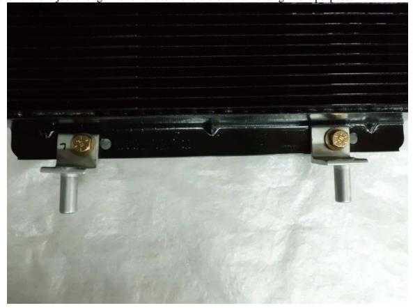
18) Install the cooler with the upper mounting brackets installed into the upper factory round grommets, reinstall the 10mm hex head mounting bolts and tighten them.
