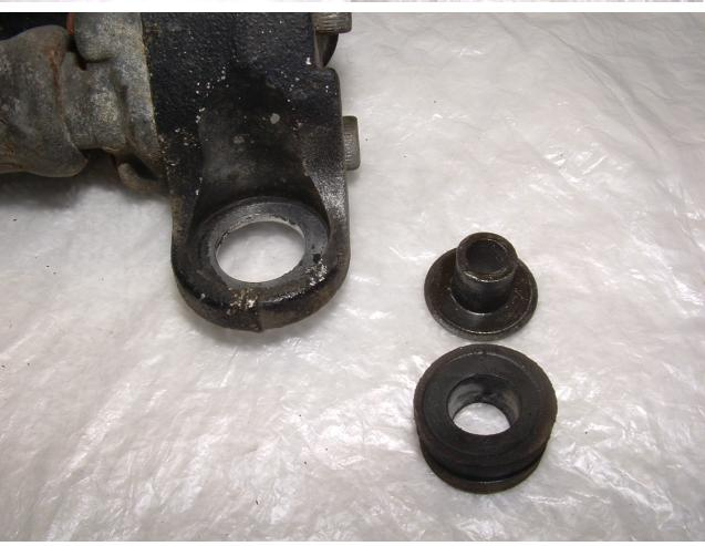
7) Remove the steel flanged sleeve insert and rubber bushing from the factory oil cooler as they will be used on the new mounting hardware. (If difficult to remove, soak in hot water to soften rubber)
