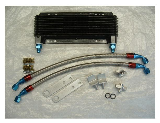
Your new oil cooler fittings are installed and torqued to the proper specification. **DO NOT tighten further or the fitting is susceptible to cracking.**
