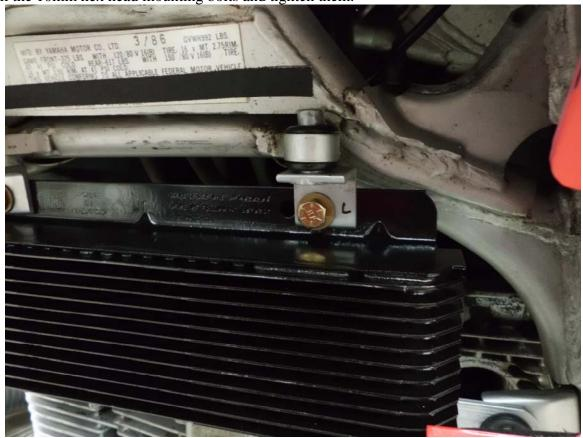
19) Tighten the <sup>1</sup>/<sub>4</sub>" upper mounting bracket bolts.
