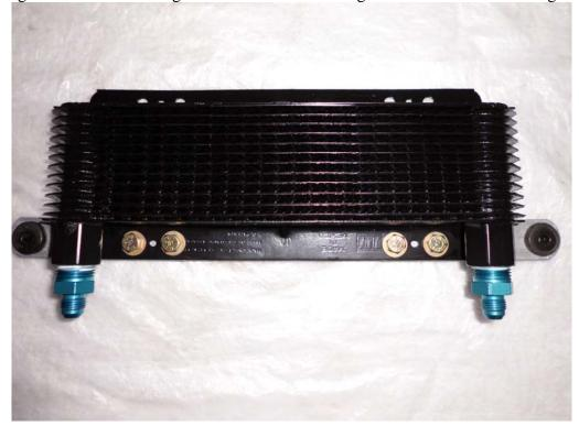
14) You will notice the upper cooler mounting flange is resting against the upper brackets. With a felt marking pen, transfer the cooler mounting hole location to the upper brackets. Designate the left and
