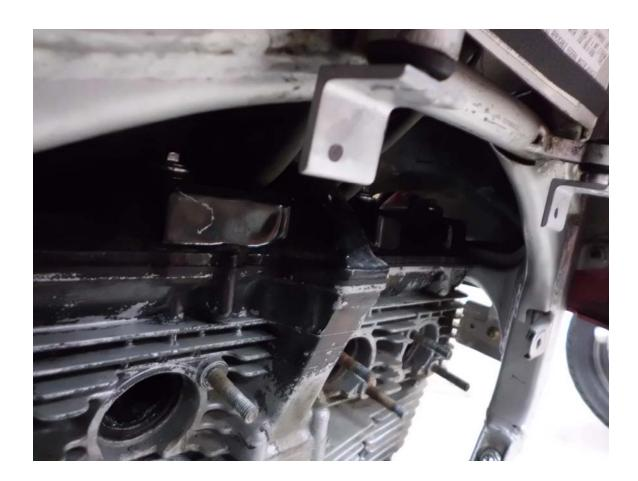
15) Remove the lower mounting bolts and cooler so the upper bracket may be removed and the hole drilled. 16) Center punch the traced hole location and drill using a 17/64" drill bit to make a hole in the upper
