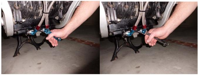
31) Use a 13/16" wrench to support the blue threaded oil cooler fitting. Using the above torqueing procedures tighten the fittings at the oil cooler; *DO NOT* allow the fitting/hose to turn or spin.
